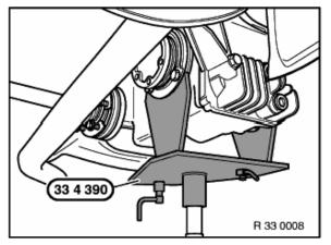
Support final drive with transmission hoist and special tool 33 4 390.
